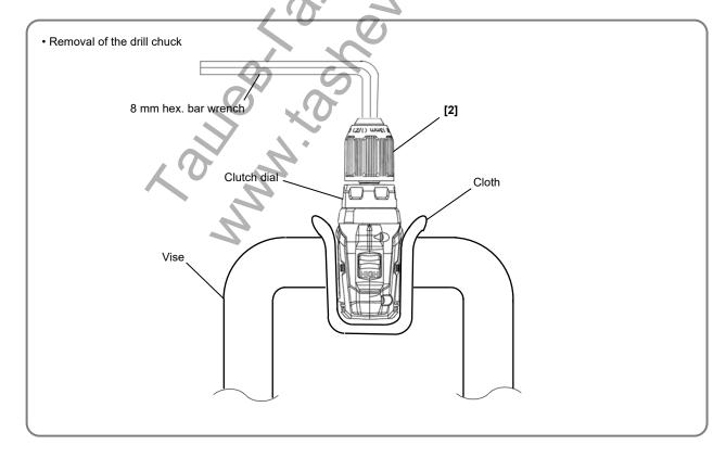
(2) Set the clutch dial to the clutch "1" position.
